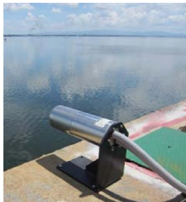
Fig. 4.1: Typical laser in its protective housing for an oil or gas terminal
